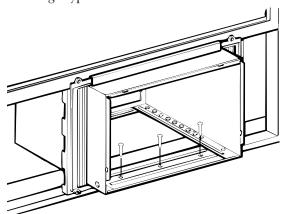
Pull the accordion panels to each window sash track. Attach them on each side to the window sash and the window stool using 4 type C screws.
